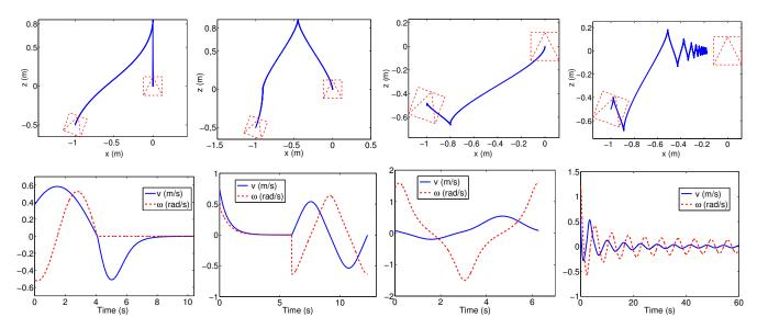
Fig. 7. Comparison of sinusoidal-input based control methods. From left to right, the four methods are: the approach presented in this paper, the method by Murray et al. [8], the method by Tilbury et al. [15], and the method due to Teel et al. [16]. The top row shows the control paths from starting location  $(-1, -0.5, -20^{\circ})^T$  for the four approaches. The bottom row displays the velocities associated to the paths on top.
