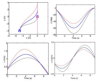
Fig. 6. Simulation results with motion drift in the sinusoidal input-based part of the control, from the initial location  $(-5, -4, -5^{\circ})^T$ . A driftless simulation is shown in a thick solid line. The results obtained adding +10% and -10% drift to both the linear and angular velocities of the robot are displayed with a dashed line and a thin solid line, respectively.
