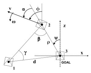
Fig. 2. Definition of the elements of our system and the geometric variables employed. '3' identifies the goal view, which serves as the global coordinate system. '2' is the robot's current location, and '1' is the location of the initial view.  $\gamma$  and  $\beta$  are angular sectors ( $\geq 0$ ) and d is the distance between the initial and target locations.
