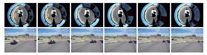
Fig. 10. Sequence of images acquired by the robot in the trajectory used in the experiments. The top row shows the images, the bottom row shows the location of the robot when the corresponding image was captured.
