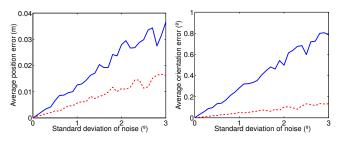
Fig. 5. Results from simulations with added Gaussian noise. Solid lines correspond to the first step of the control; dashed lines correspond to the second. The average position (left) and orientation (right) errors at the end of each step are displayed.
