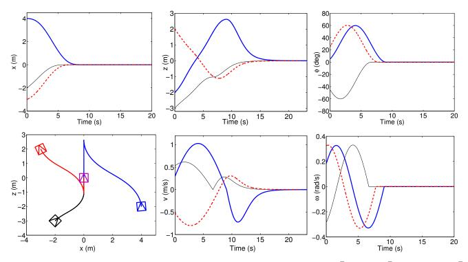
Fig. 4. Three sample robot trajectories for the sinusoidal input-based control, from starting locations  $(4, -2, 5^{\circ})^T$ ,  $(-3, 2, 25^{\circ})^T$  and  $(-2, -3, -45^{\circ})^T$ . The evolutions of the state variables x (left), z (center) and  $\phi$  (right) are displayed in the top row. The second row shows the robot paths (left) for each trajectory, the linear velocity (center) and the angular velocity (right).
