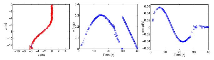
Fig. 11. Results from the experiment with the real robot. Estimation of the position (marked with triangles) along the trajectory superimposed on the odometry, which is shown in a solid line (left). Computed linear velocity (center) and angular velocity (right).
